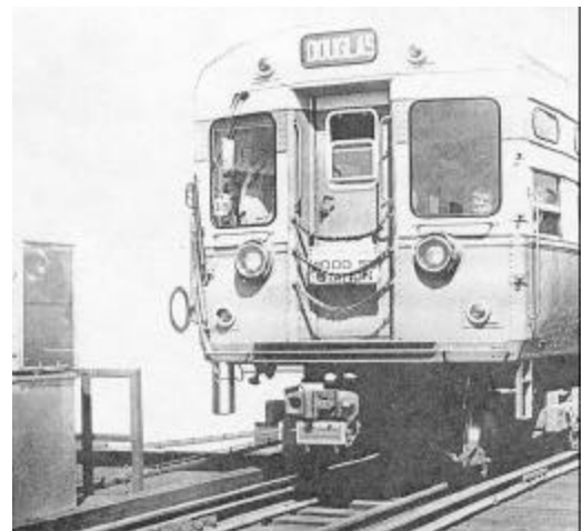
A Douglas train of 6000-series cars. Note the circular coil on the bottom left: it emits a radio signal that triggers the proper alignment for the train at Paulina Junction, where this 1953 photo was taken. The sign on the chains indicates that it will stop a Wood Street station, a "special service" station between 18th and Hoyne, now long demolished.
